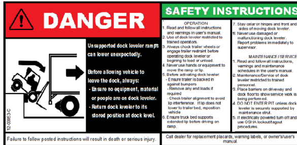
2 SEL-12-00053-C EOD Danger Label (Place on exterior side of left bumper & interior side of right bumper Typ. of two)
