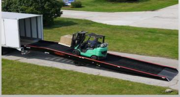
Copperloy specializes in mobile yard ramps . Yard ramps are a perfect solution for forklifts to get from ground level to dock or truck height. Ramps have a capacity range from 16,000 to 35,000 pounds. Some models are in stock for immediate shipping. We also have rentals available in our 20,000 pound capacity mobile ramps.
