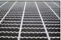
Deck Grating—Constructed of electroforged serrated steel for superior strength. Grating bearing bars are 2 1/4" thick for durability in the roughest of applications. Bars are spaced 1" apart to resist clogging of debris and to insure al all-weather high traction running surface.
