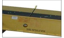
Pump—Hydraulic hand pump quickly adjusts top end of ramp with the bed of the vehicle or loading dock. The handle is stored out of the way when not in use.
