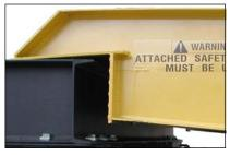
15" Lip—Deep overlap of frame at high end is assurance that the ramp rests firmly on the carrier body or dock floor. Eight foot long safety chains and hooks are provided for added security. When correctly rigged, chains join the ramp and vehicle into a single unit.
